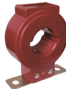
MODEL: FU-LV42 500/5A 7.5VA CLASS 0.5 600/5A 10VA CLASS 0.5
